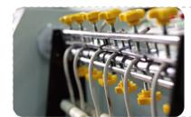
Bend-resistant cable, withstanding hundreds of thousands of bending tests
