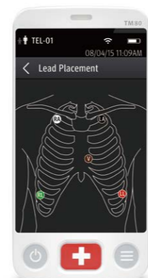
ECG lead-off guide, helps nurse locate the lead that is not properly connected.
