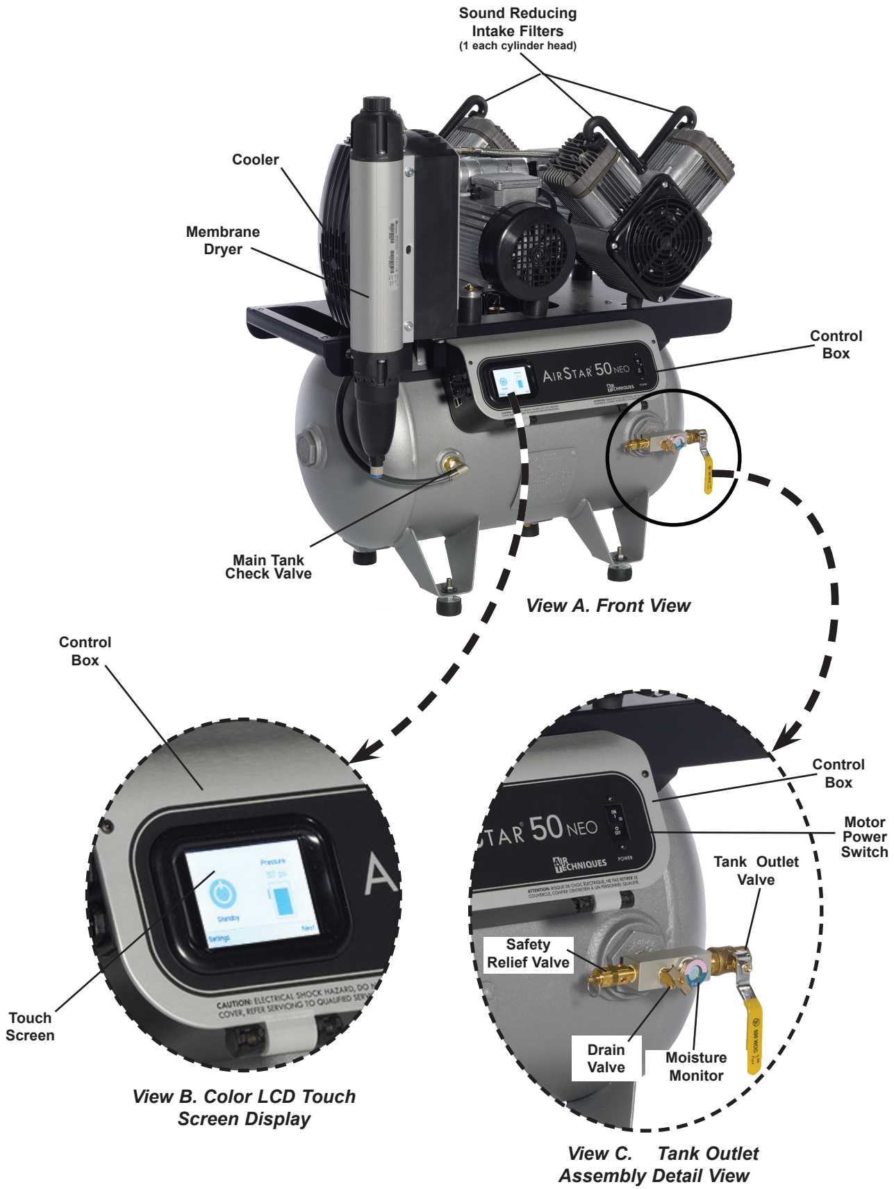
Figure 1. AirStar NEO Parts Location
