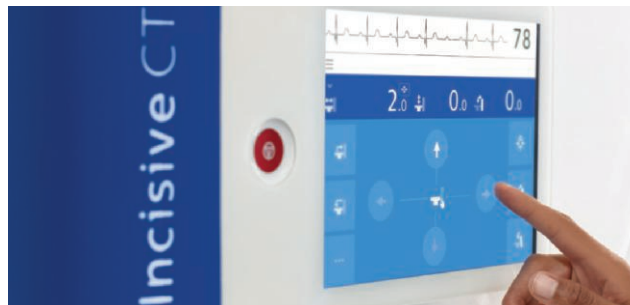
Easily move the couch by touching the panel screen and swiping in the direction of desired movement.
