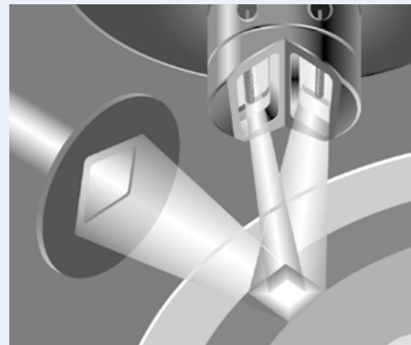
Principle of the "mixed" focus spots, here with a diagram
