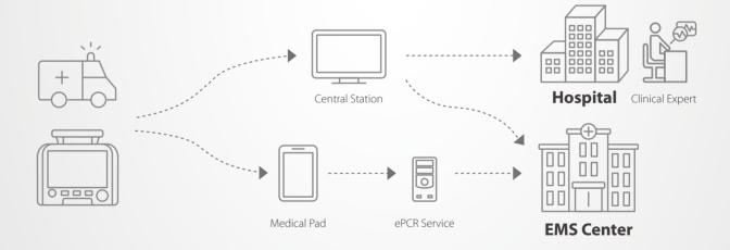
The patient's ventilation and monitor data during transport can be transmitted to the hospital in real-time. The medical staff can remotely monitor the patient's ventilation and vital signs through the hospital's CMS(central monitoring system) or ePCR system to formulate timely treatment plan.
