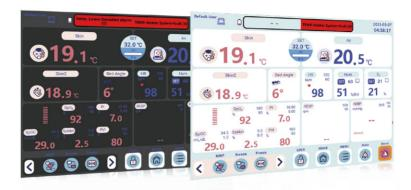
■ LCD display: 12.1-inch TFT color LCD touch screen, night mode can be set to reduce the impact of light stimulation on newborns;
