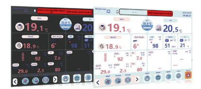
■ LCD display: 12.1-inch TFT color LCD touch screen, night mode can be set to reduce the impact of light stimulation on newborns.
