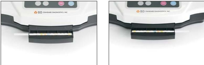
[Fig 3.7] Strip Loading after set up stray
